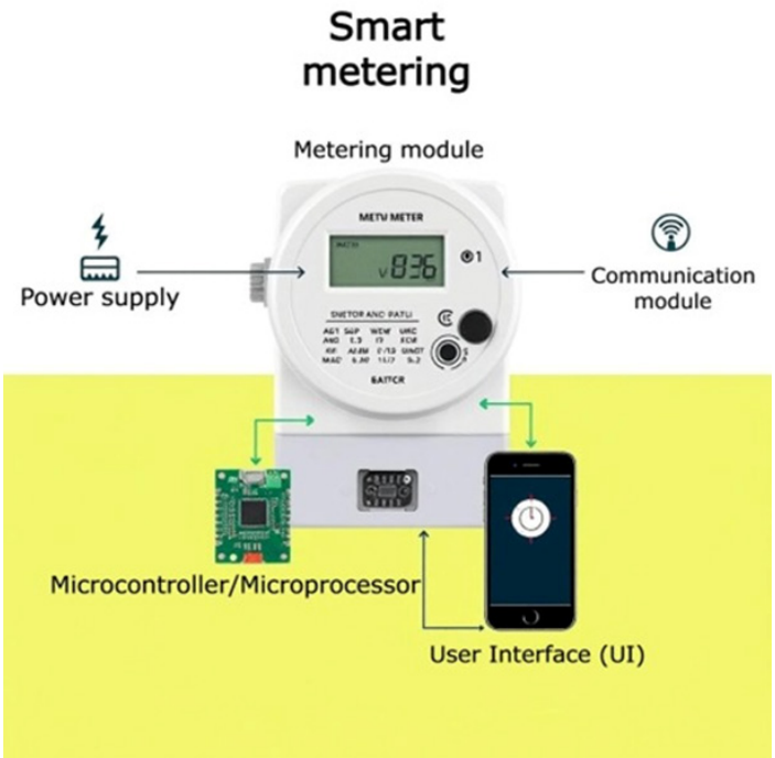
Figure 1: Key components of Smart meter
