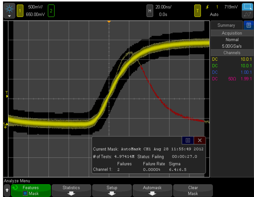
Figure 5. Mask tests make it easy to observe when a signal fails the QA process
