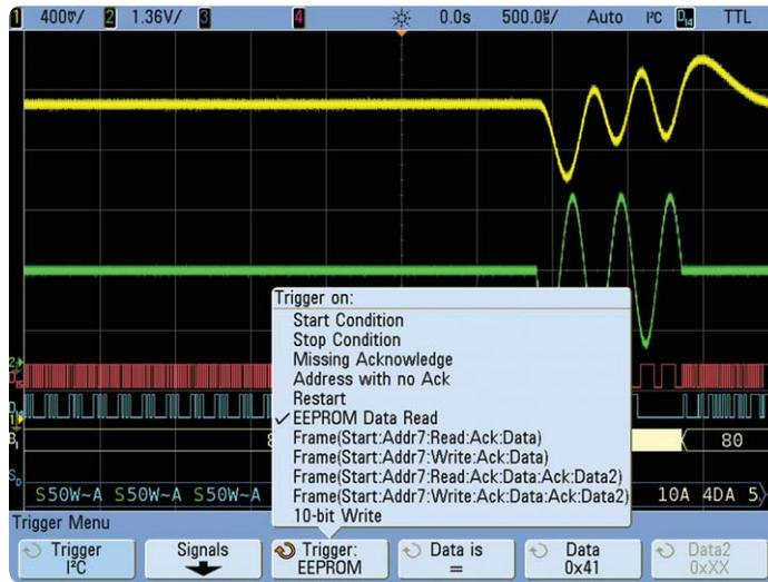
Figure 12. Triggering on a 3-cycle chirp with I<sup>2</sup>C triggering and decode in an Agilent MSO.
