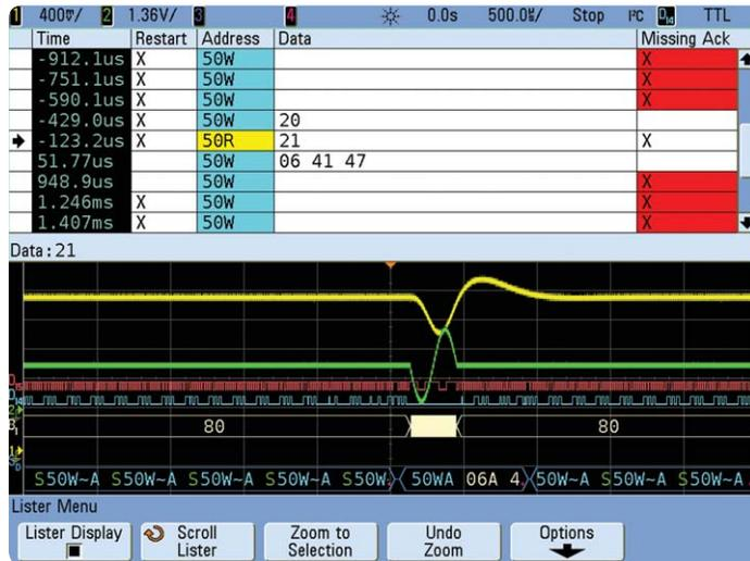
Figure 13. Triggering on a 1-cycle chirp with I<sup>2</sup>C triggering and decode in an Agilent MSO.
