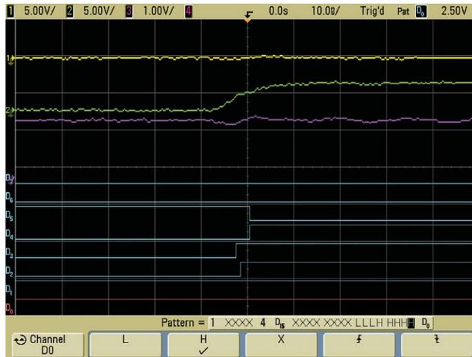
**Figure 5. With minimum time-qualification, the Agilent MSO does not trigger on unstable conditions.**
