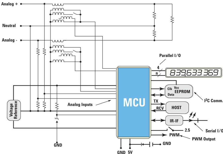
Figure 2. Typical MCU-based embedded design
