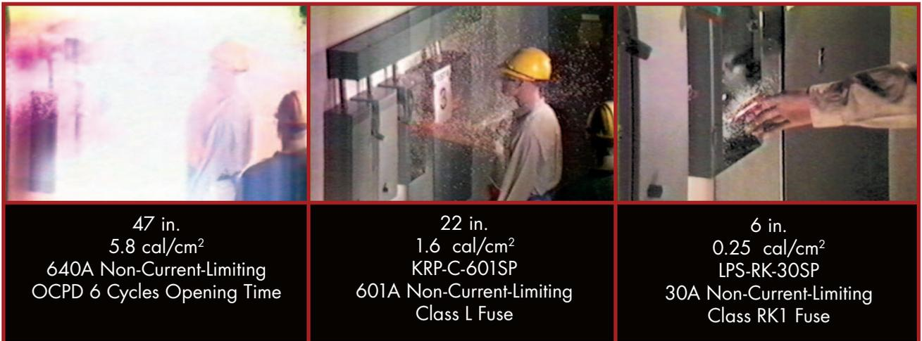
**Figure 2.** The use of overcurrent protective devices has a strong impact on the magnitude and duration of arc flash faults.
