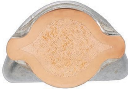
**Figure 1.** Crimping tools with circular crimping dies result in a solid copper mass for greater conductivity.
