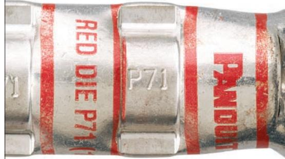
**Figure 2.** Circular crimping dies emboss the die index number into the lug during crimping for easy inspection.
