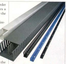
According to NFPA 79, the maximum permitted wire fill amount for wiring duct is 50 percent. Most manufacturers supply a wire-fill chart in their catalogs and Web sites based on the 50-percent fill rule.
