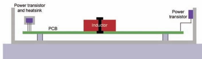
Figure 1: Construction of typical industrial AC/DC power supply
