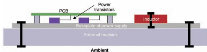
Figure 2: Construction of BCC Series power supply for harsh environment applications
