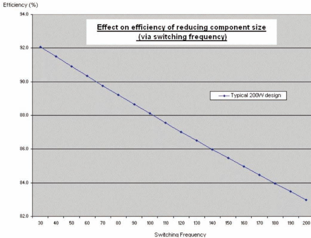
Figure 1: Effect on efficiency of reducing component size by increasing switching frequency
