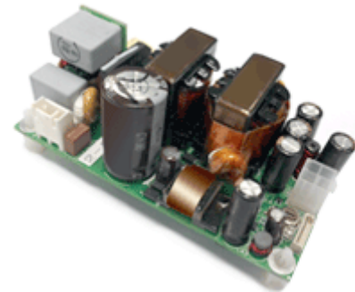
Large Capacitors in a Power Supply
