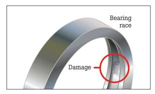
A failed bearing has increased drag, emits more heat, and has lower efficiency because of a mechanical, lubrication, or wear problem. Bearing failure can be caused by several things:
