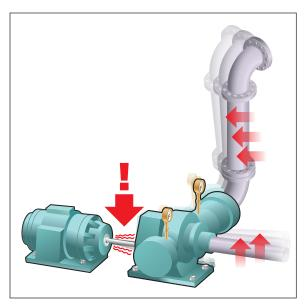
Pipe strain refers to the condition in which new stresses, strains, and forces, acting on the rest of the equipment and infrastructure transfer backward onto the motor and drive to induce a misalignment condition. The most common example of this is in simple motor/pump combinations, where something applies force to the pipeworks such as:
