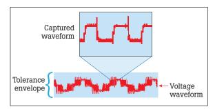
Variable frequency drives employ a pulse width modulation (PWM) technique to control the output voltage and frequency to a motor. Reflections are generated when there is an impedance mismatch between the source and load. Impedance mismatches can occur as a result of improper installation, improper component selection or equipment degradation over time. In a motor drive circuit, the peak of the reflection could be as high as the DC bus voltage level.
