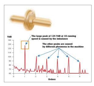
Imbalance is a condition of a rotating part where the center of mass does not lie on the axis of rotation. In other words, there is a "heavy spot" somewhere on the rotor. Although you can never completely eliminate motor imbalance, you can identify when it is out of normal range, and take action to rectify the problem. Imbalance can be caused by numerous factors, including:
