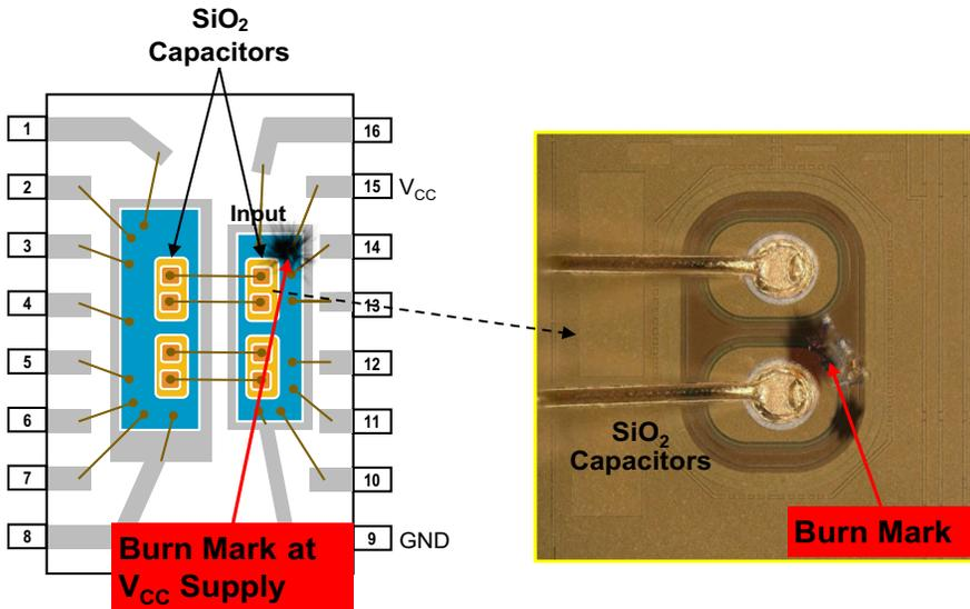
Figure 7 shows that the SiO<sub>2</sub> capacitor is damaged at the input IC and the insulation capability of the isolator is compromised. The insulation circuit being integrated on the same chip, along with the input circuitry in a monolithic process and a thin DTI, is the obvious reason for the insulation failure. This result shows that the single point failure of the power supply can damage the capacitive insulation barrier. This damage can lead to electric shocks and compromise safety.
