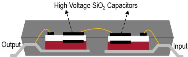
The construction of a gate driver using capacitive isolation in a two-chip module is shown in Figure 4. The input and output ICs have isolation capacitors to increase the high-voltage capability. As this construction is a monolithic process, the input IC of the gate driver consists of the power supply circuit, PWM control circuit, and  $\text{SiO}_2$  capacitor in a single chip.
