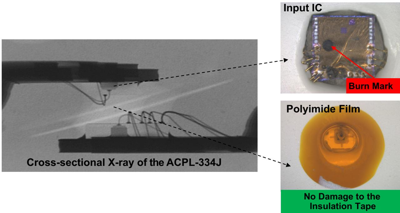
The gate driver using capacitive insulation shows very high leakage current that exceeds the limit of the high-voltage tester. A failure analysis was conducted to see the extent of the damage that caused the high leakage current.
