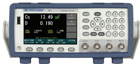
The 891 is a compact, precise, and versatile LCR meter capable of measuring inductors, capacitors and resistors at DC or from 20 Hz to 300 kHz, at both low and high impedance ranges. A large color display with all important parameters and measurement visible on one screen makes this meter easy to operate. The outstanding performance of the 891 makes it an invaluable tool for production, quality control, and R&D.
