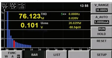
The parameters of each harmonic measured can be displayed in a bar chart.
