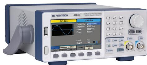
The 4060B Series Dual Channel Function/Arbitrary Waveform Generators are capable of producing precise sine, square, triangle, pulse, and arbitrary waveforms. The intuitive touchscreen display simplifies control of many features including extensive waveform modulation schemes, linear/logarithmic sweep, burst mode, and variable DC offset.
