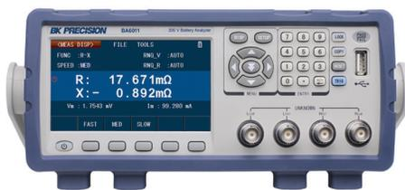
The BA6010 Series Battery Analyzers use a 1 kHz AC constant current source to measure the battery's impedance expressed by 11 different measurement functions. With a basic voltage and impedance accuracy of 0.1% and micro-ohm resolution, these instruments are well-suited for analyzing a wide range of battery types and configurations in the lab, quality control and manufacturing environments.
