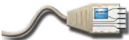
A 1-Wire device and wired sensor with DB9 connector interface to the instrument.
