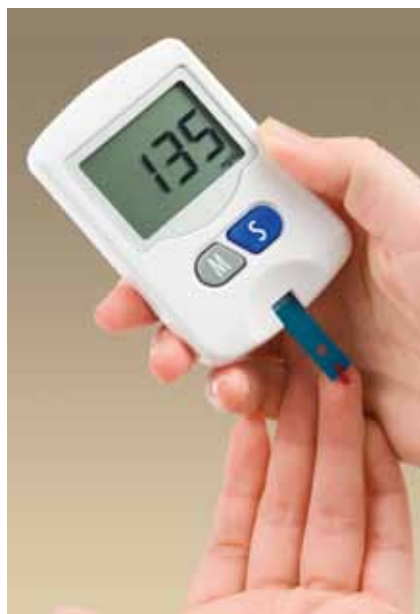
Electrochemical blood glucose meter
